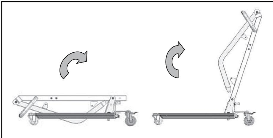
3. Pull the mast, boom, and spreader bar to an upright position, as shown above.
